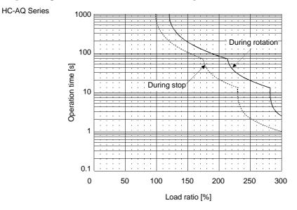
Fig 11.1 Electronic Thermal Relay Protection Characteristics
